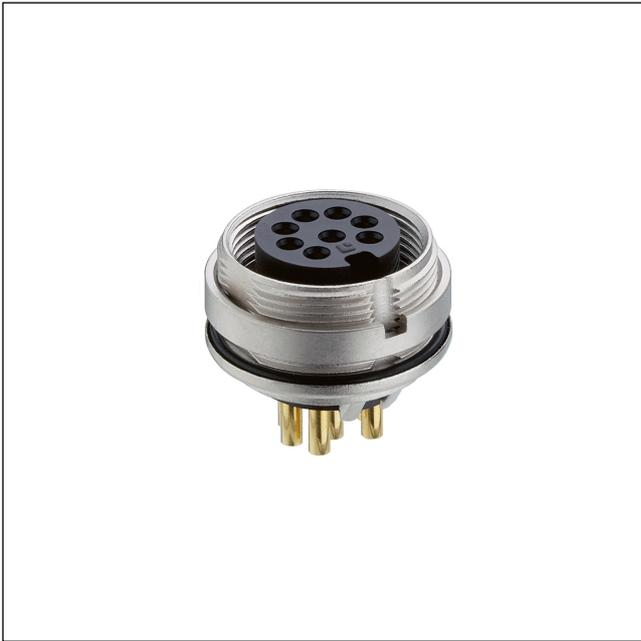
SWUM™ chassis socket acc. to IEC 61076-2-106 and AISG specification, IP68/67, with threaded joint and solder terminals, for back side mounting
